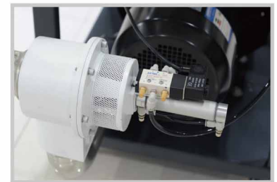
Vacuum breaking valve
