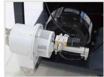
Vacuum breaking valve
